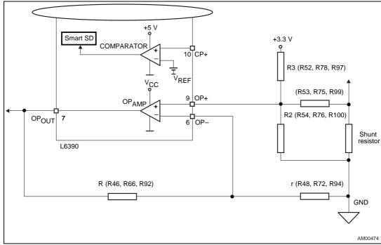
Figure 12. Three-shunt configuration
