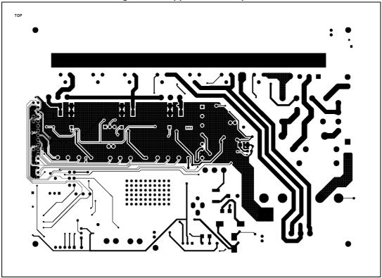
Figure 19. Copper tracks - bottom side
