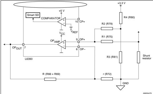
Figure 13. Six-step current sensing configuration
