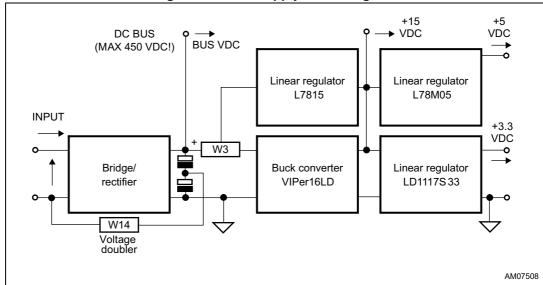
Figure 9. Power supply block diagram
