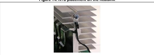
Figure 14. NTC placement on the heatsink
