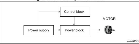
Figure 2. Motor control system architecture
