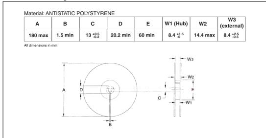
Figure 5. Seven-inch reel mechanical dimensions.
