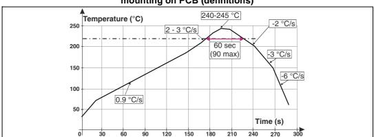
Figure 10. ST ECOPACK<sup>®</sup> recommended soldering reflow profile for Flip-Chip mounting on PCB (definitions)
