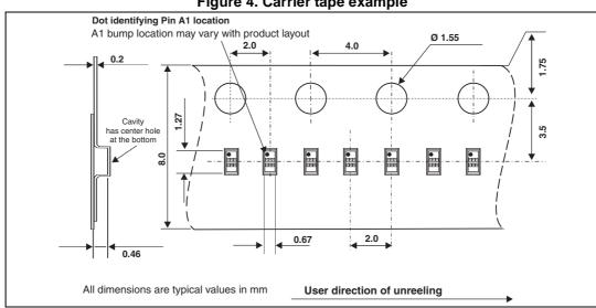
Figure 4. Carrier tape example
