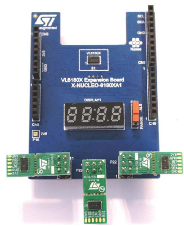
Figure 4. Connections of VL6180X satellite boards
