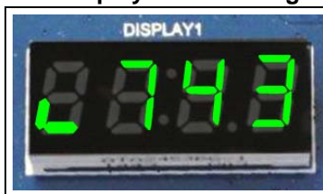
Figure 26. Left digit of the display if ambient light value below 1000 Lux
