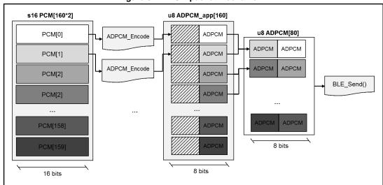
Figure 6: ADPCM packet mechanism
