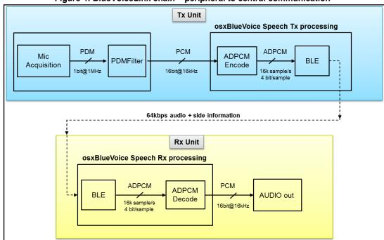
Figure 4: BlueVoiceLink chain - peripheral to central communication
