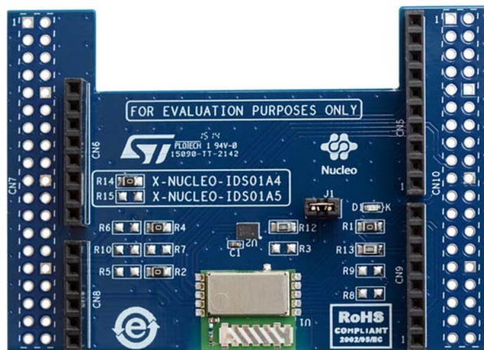
Figure 13. X-NUCLEO-IDS01Ax expansion board
