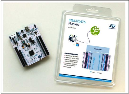
Figure 2. NUCLEO-L476RG Nucleo board
