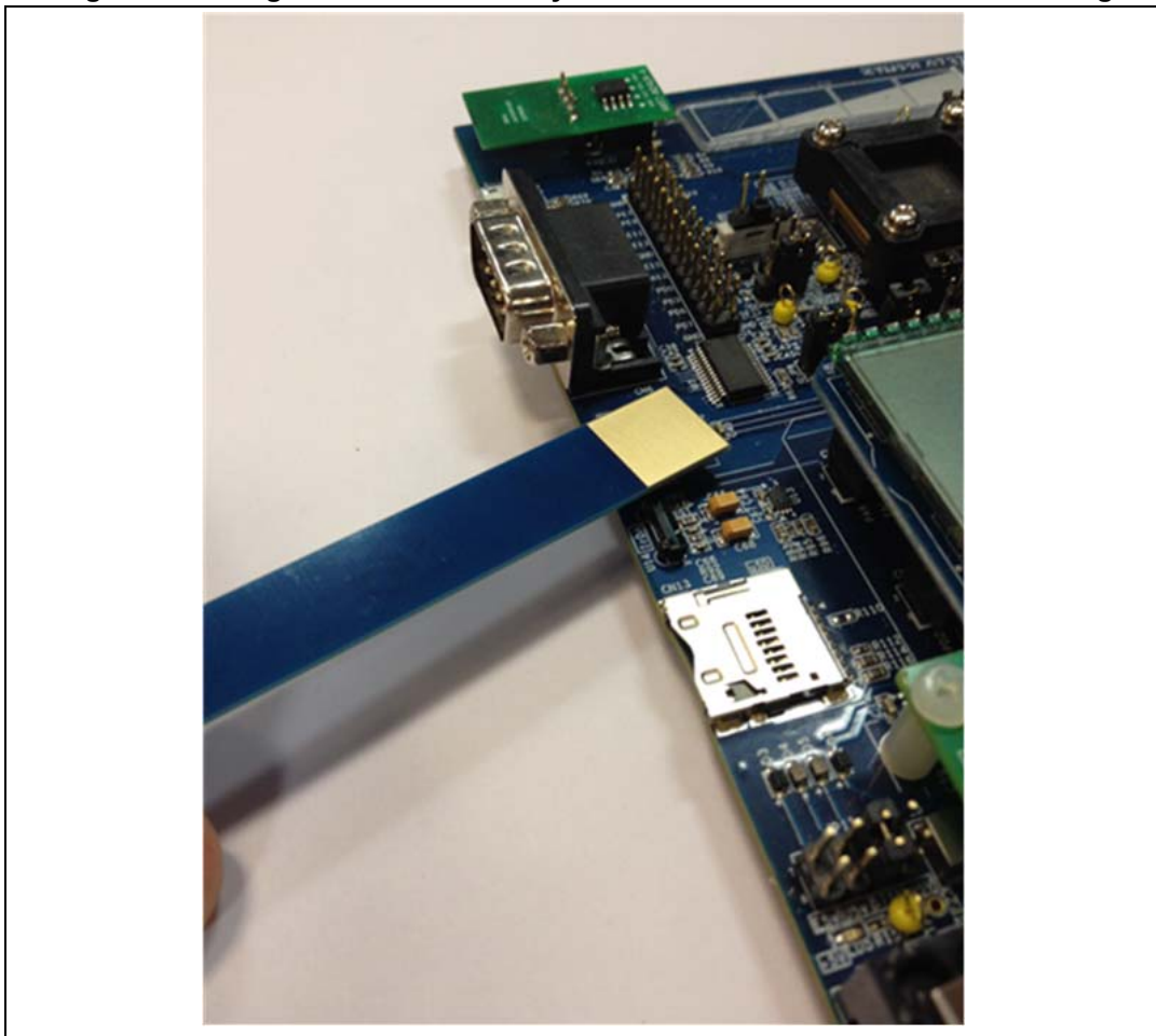
Figure 15. Using detection accessory board MB1199 with LC sensor metering
