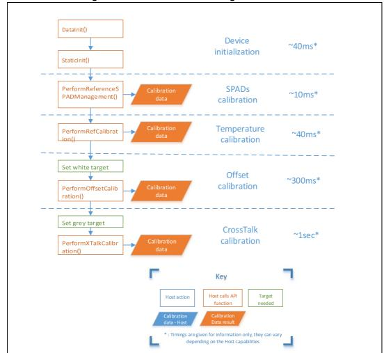
Figure 2. Customer manufacturing calibration flow
