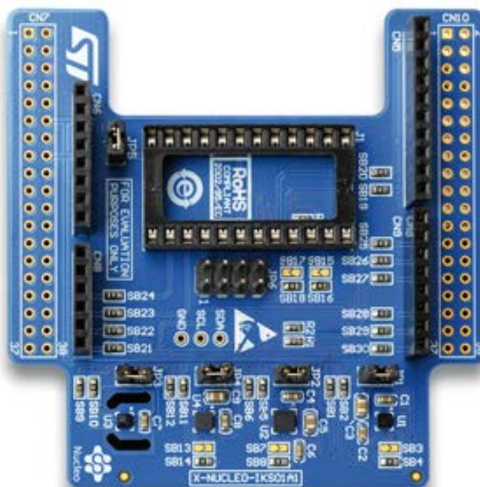
Figure 60. X-NUCLEO-IKS01A1 expansion board
