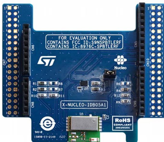
Figure 59. X-NUCLEO-IDB05A1 expansion board
