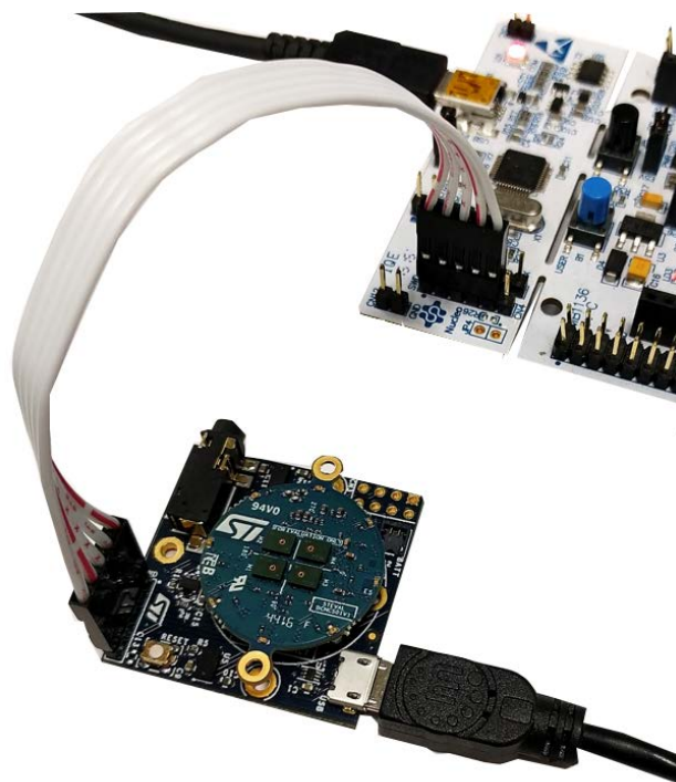
Figure 73. BlueCoin-STM32Nucleo: SWD connections with 5-pin flat cable
