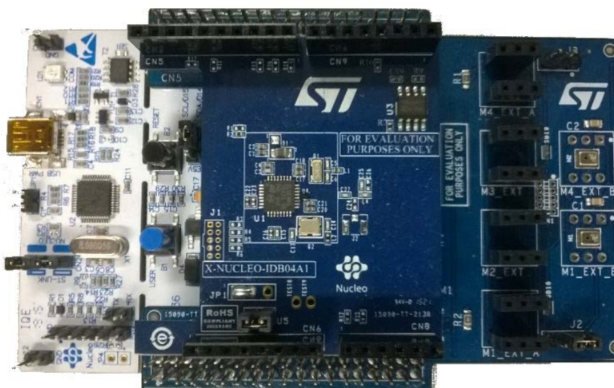
Figure 70. STM32 Nucleo plus X-NUCLEO-CCA02M1 plus X-NUCLEO-IDB04A1 boards
