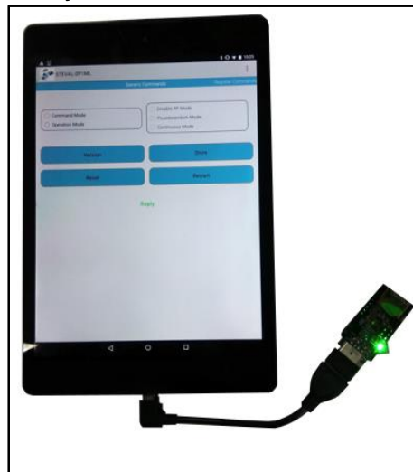
Figure 3: Physical USB connection of SP1ML module
