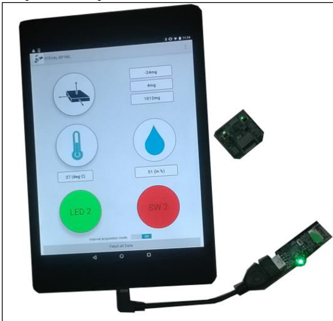
Figure 23: SP1ML Dongle connected to mobile and STEVAL-IDI005V1 in active mode.
