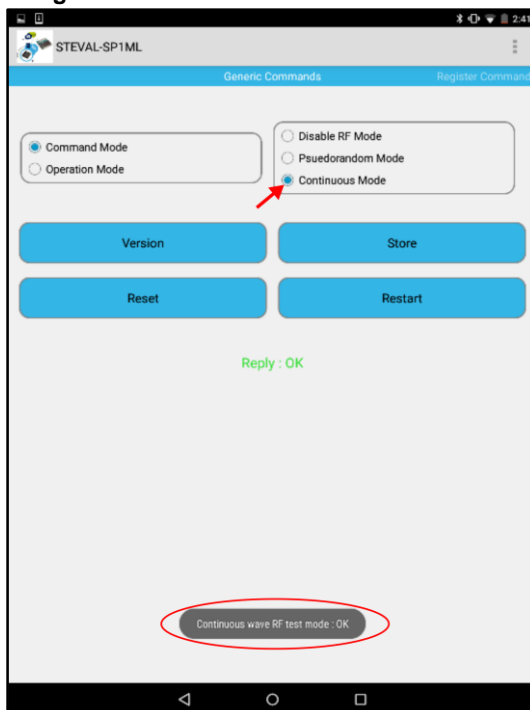
Figure 11: Continuous wave RF test mode
