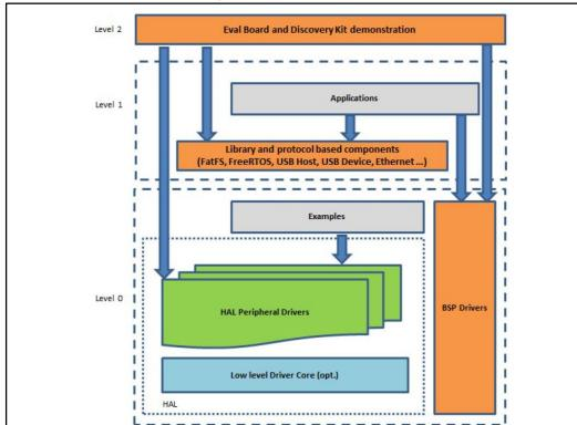
Figure 1: Firmware architecture
