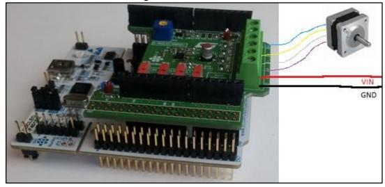
Figure 6: Board connections
