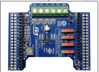
Figure 5: X-NUCLEO-IHM06A1 low voltage stepper motor driver expansion board
