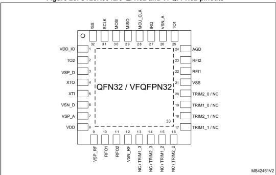
Figure 28. ST25R3912/3 QFN32 and VFQFPN32 pinouts<sup>(1)</sup>
