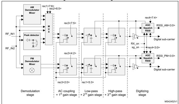
Figure 4. Receiver block diagram
