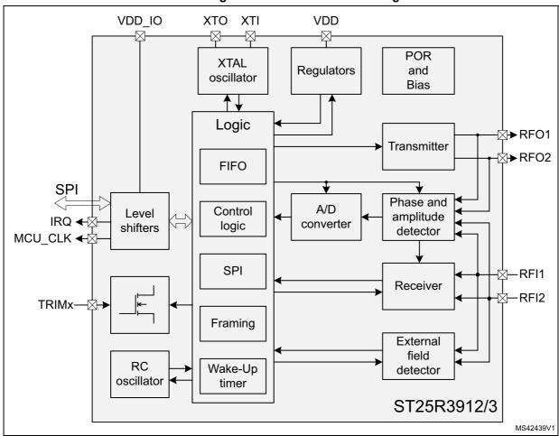
Figure 1. ST25R3912/3 block diagram
