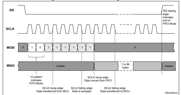
Figure 13. SPI communication: reading of FIFO
