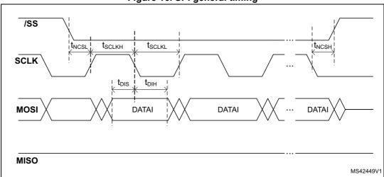
Figure 17. SPI read timing
