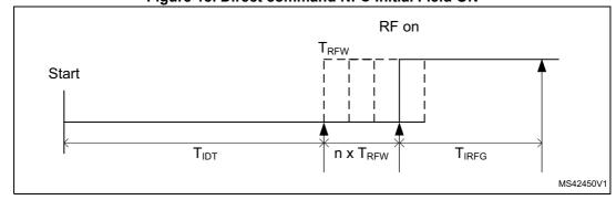
Figure 18. Direct command NFC Initial Field ON
