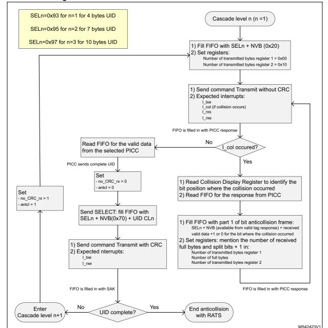
Figure 22. Flowchart for ISO14443A anticollision with ST25R3912/3
