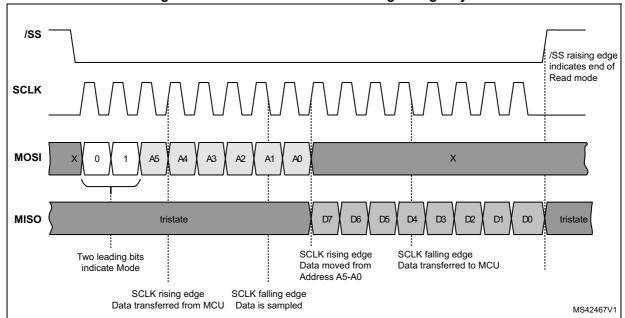
Figure 11. SPI communication: reading a single byte
