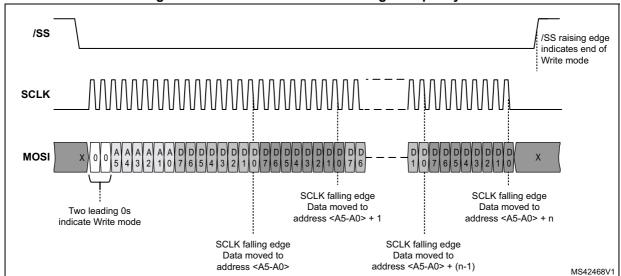
Figure 10. SPI communication: writing multiple bytes
