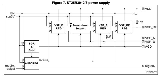
*Figure 7* shows the building blocks of the ST25R3912/3 power supply system and the signals that control it.
