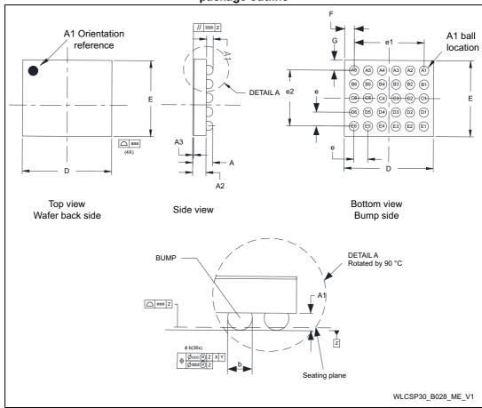
Table 104. WLCSP30 30-ball, 3.065 x 2.865 mm, 0.5 mm pitch wafer level chip scale mechanical data
