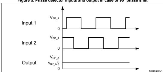
Figure 5. Phase detector inputs and output in case of 90° phase shift
