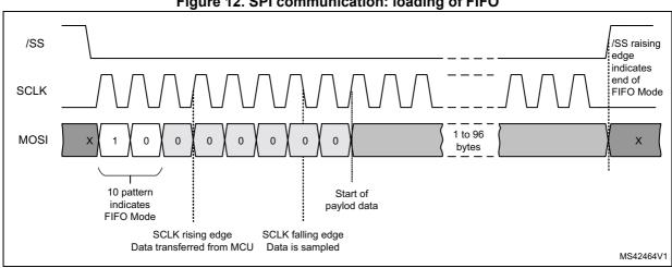
Figure 12. SPI communication: loading of FIFO
