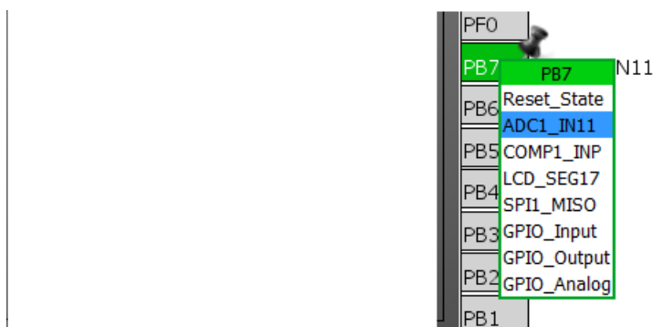
Figure 61. Modifying pin assignments from the Chip view
