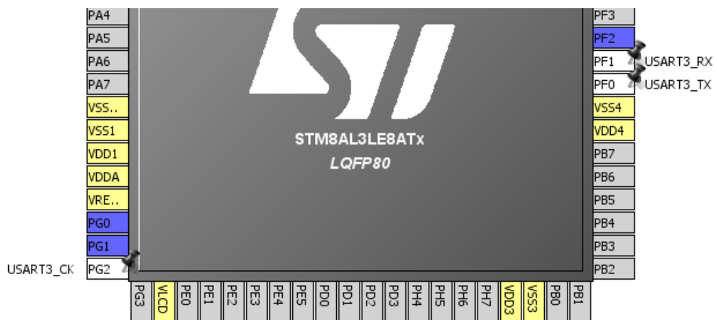
Figure 64. Example of remapping with destination pin ambiguity
