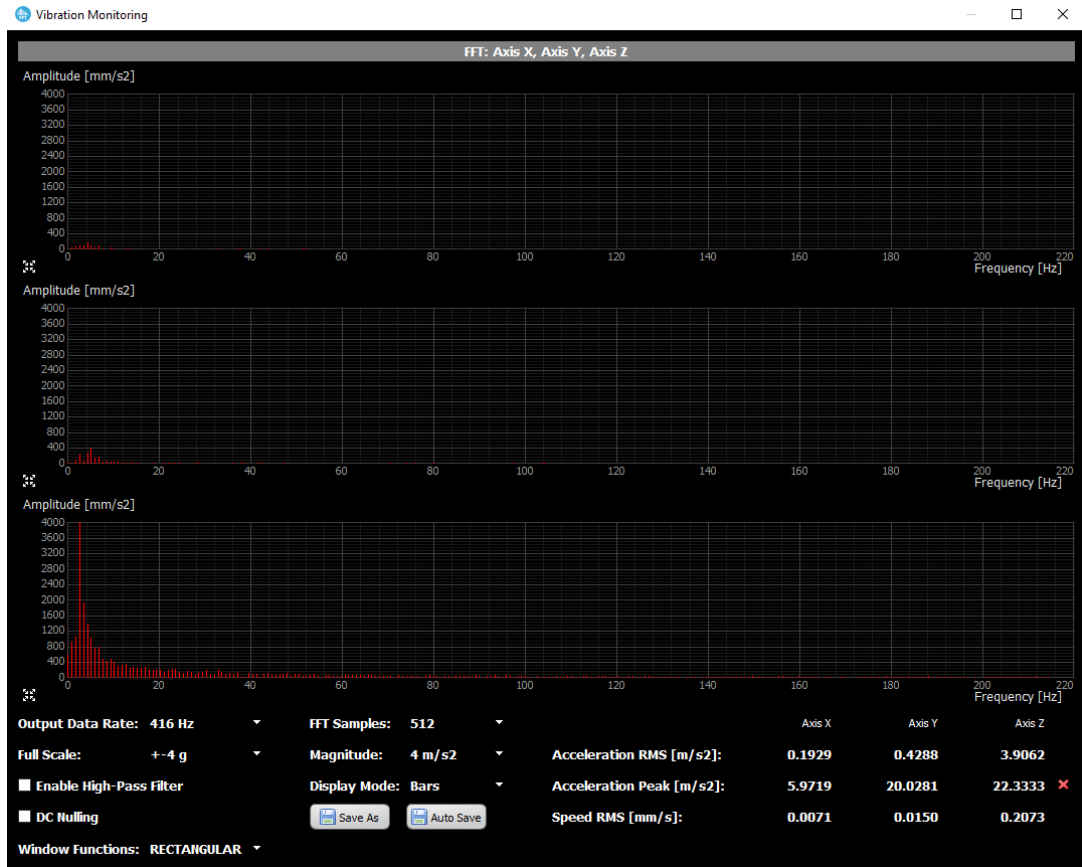
Figure 15. Vibration Monitoring - Unicleo-GUI spectrum plots, settings and calculated results
