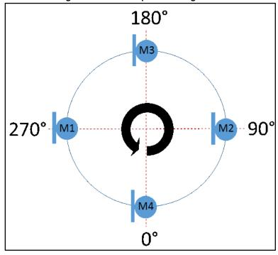
Figure 2: Four-microphone arrangement
