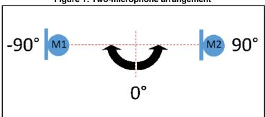
Figure 1: Two-microphone arrangement
