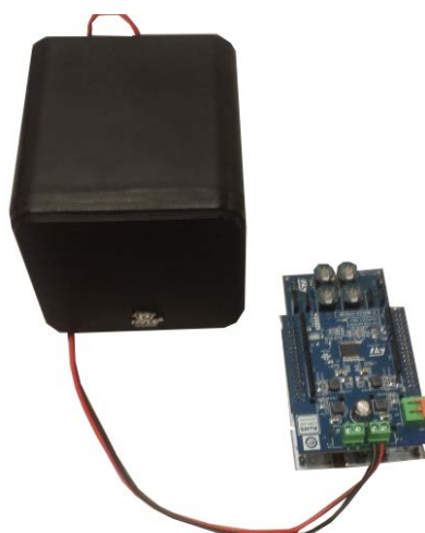
Figure 10. Loudspeaker connected to the board stack
