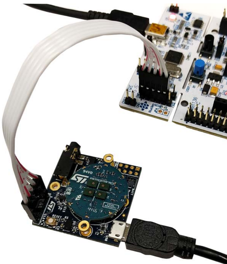
Figure 18. SWD connections with 5-pin flat cable
