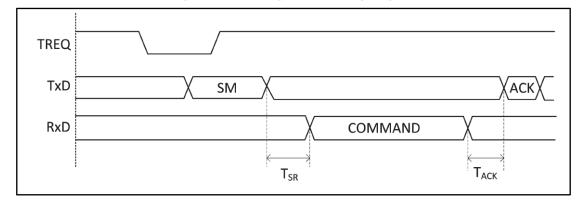
Figure 2: TREQ negotiation timing diagram
