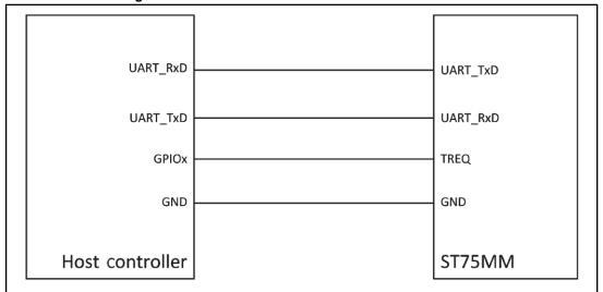
Figure 1: Host controller to ST75MM connection scheme
