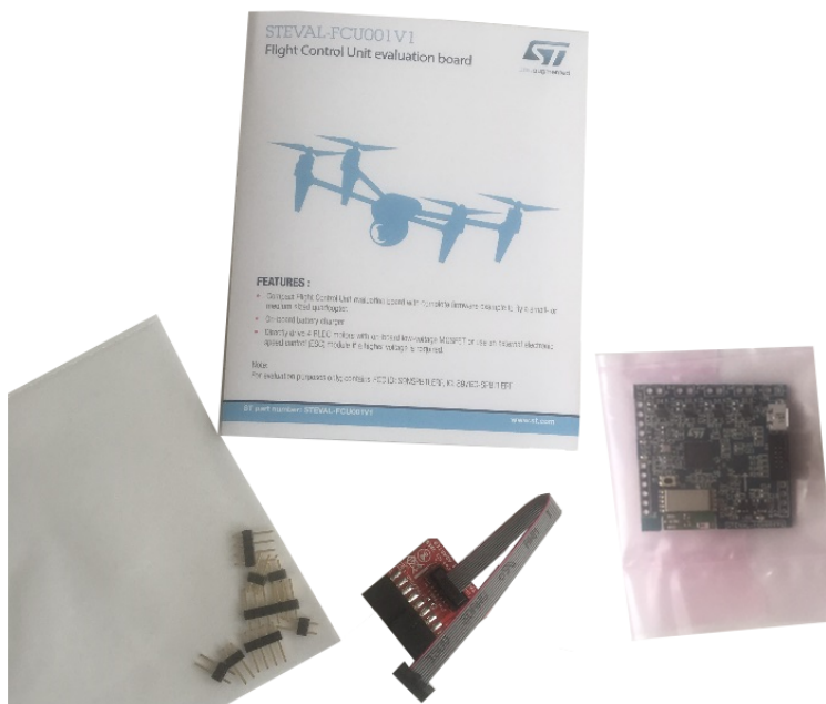
Figure 2. STEVAL-FCU001V1 evaluation board: package contents
