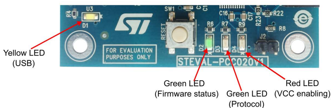
Figure 7. STEVAL-PCC020V1 interface board status LEDs
