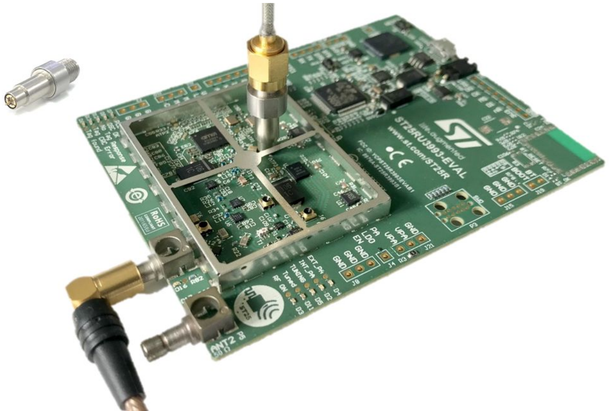
Figure 14. Connecting to the RF test points with the SMB adapter
