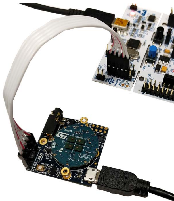
Figure 35. BlueCoin-STM32Nucleo: SWD connections with 5-pin flat cable
