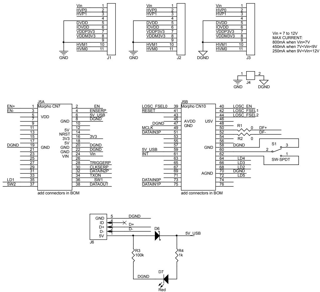
**Figure 15. STEVAL-IME014V1 schematic diagram**
