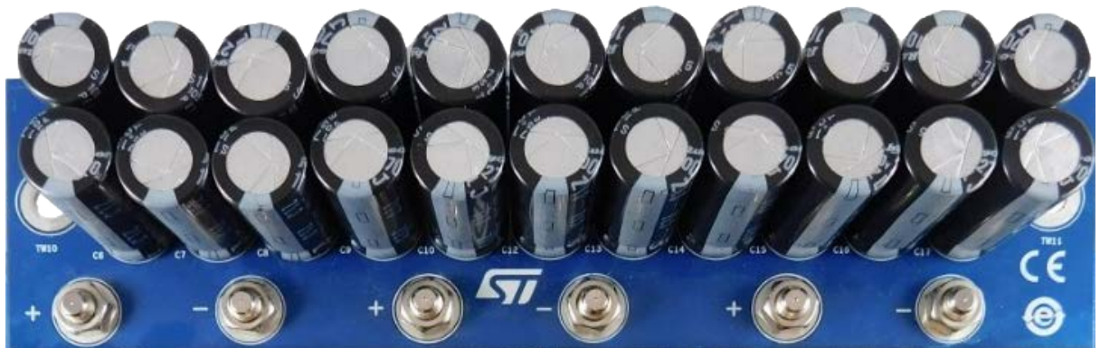
Figure 7. STEVAL-CTM005V1 bus link capacitor board
