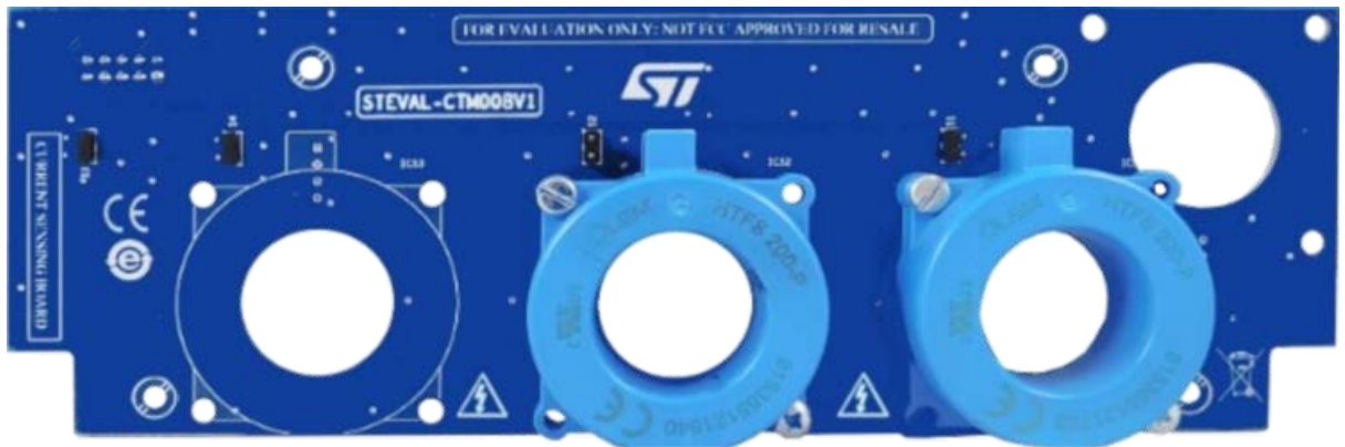
Figure 8. STEVAL-CTM008V1 current sensing board
