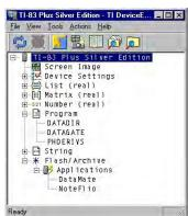
5. The program should now be loaded into your calculator. To confirm this, press on the calculator to display the loaded applications.
