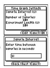
value by pressing Cear or by pressing and DEL. You can also type over the current value by pressing and entering a new sample interval. Note that EasyData allows only certain sample intervals. If you enter a sample interval that EasyData does not support, an error message will appear and a sample interval will be chosen for you.
