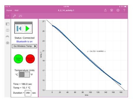
Possible results from project evaluation. The Go Wireless Temp sensor was placed in the bottle shown above and put in a refrigerator for 3 minutes. Although this data is not perfectly linear (nor should it be), a linear regression may be a good method of analysis and an appropriate level of mathematical modeling for students.
