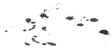
Students will repeat the procedure twice more, moving the pipette to slightly different locations but maintaining a height of 10 cm. Students calculate the average diameter of the spatters that fell from 10 cm, and record it in the Evidence Record. Students replace the white paper with a clean sheet, and then repeat steps 1 - 3 for each remaining height in the Evidence Record.
