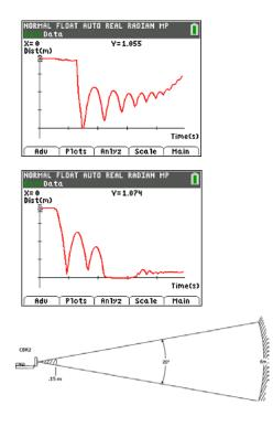
• The path of the CBR 2 beam is not a narrow, pencil-like beam, but fans out in all directions up to 10° in a cone-shaped beam. The CBR 2 can handle distances from 0.15 meters to about 6.0 meters.
