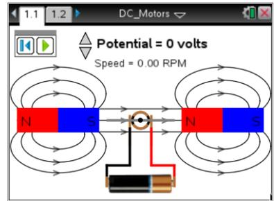
As you explore the motor you will examine the relationship between the voltage of the power supply and the speed of the rotor. A DC motor is a collection of parts connected in such a way as to have a spinning rotor that will then be used to do work.
