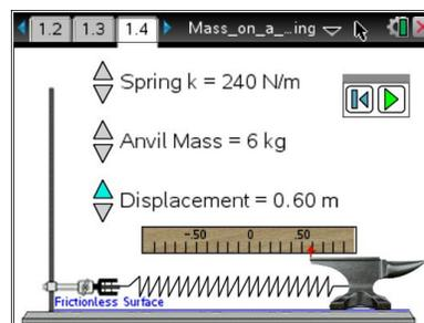
In the simulation, students set the anvil's mass ( $2 \text{ kg} \leq m \leq 10 \text{ kg}$ ), the spring constant of the spring ( $40 \text{ N/m} \leq k \leq 300 \text{ N/m}$ ), and the initial position of the anvil ( $-1 \leq x_i \leq 1 \text{ m}$ ).
