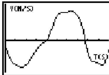
14. The graph is generated by walking away from the CBR™ at a constant rate, then walking toward the CBR at a constant rate, and then walking away for a second before turning around.
