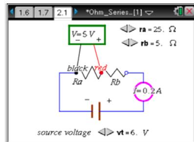
Polarity: all circuit components have a polarity designated positive (+) and negative (-). The polarity is determined with reference to the source; from any component end go straight back to the source to find the polarity. To measure voltage across a resistor, drag the ends of the voltmeter wires to the ends of the resistors. It will only work if it is connected with the correct polarity.
