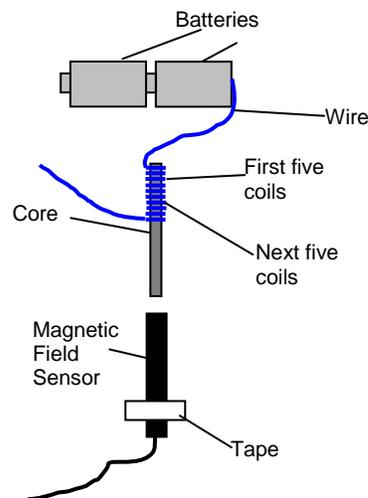
Step 9: Students should repeat steps 6–8 until they have wrapped the wire along the entire length of the core. For each data point, students should use the number of turns, or coils, on the core as the data value.
