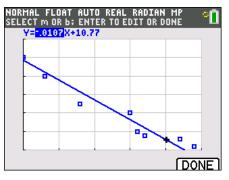
Once the line is drawn, students can use the left and right arrow keys ( $\blacktriangleleft$  and  $\triangleright$ ) to select and adjust the *y*-intercept or the slope and type in new values for the equation. When the students have a satisfactory manual fit line, have them record the equation of the line rounded to 2 or 3 decimal places. The equation is stored in the  $\gamma$ - editor.
