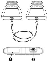
The USB port is located on the top of the TI-Nspire<sup>™</sup> CX handheld on the right side when holding the handheld with the screen facing you.
