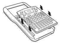
• Push the keypad firmly into place. You will hear a click and the switch on the back of the keypad is in the locked position.
