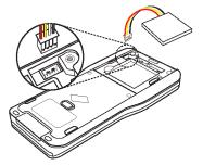
4. Thread the wire into the case to secure it. Insert the rechargeable battery into its compartment.
