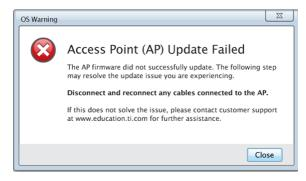
To resolve the problem, disconnect and reconnect any cables connected to the access point, and the software will automatically start the update process. If this does not resolve the issue, contact Customer Support.
