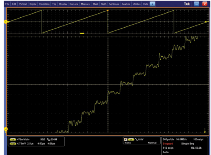
Figure 19. Zoomed display of the same high-resolution ramp signal, based on a large number of averages, showing significantly higher vertical resolution.
