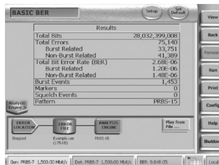
Error Statistics View showing link performance in terms of bit and burst occurrences.
