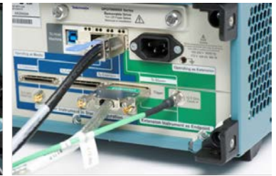
UltraSync connection on instrument with Extension role
