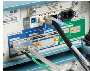
UltraSync connection on instrument with Master role
