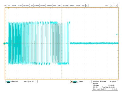
9. Adjust the scope Horizontal scale so that one complete packet is displayed
