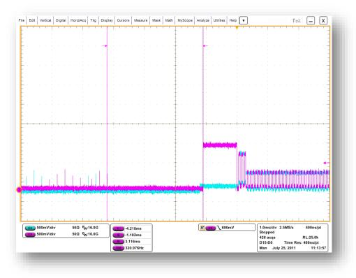
Figure 22: Device Chirp-K in Response to Reset from High-Speed (EL\_27)
