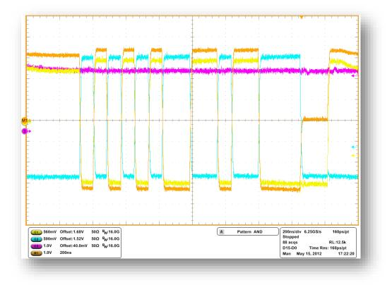
Figure 37: Full Speed Signal Quality trigger
