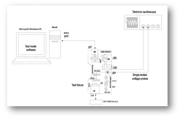
Figure 14: Equipment Setup for Suspend Measurement
