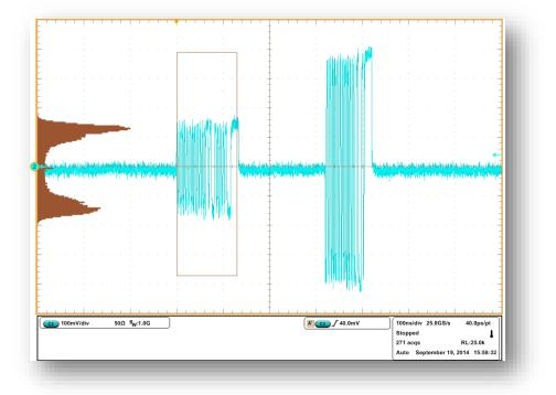
Figure 33: Measuring Differential Voltage Level - Zero to Positive Peak
