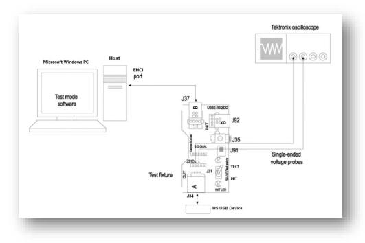
Figure 23: Equipment for Reset from Suspend Measurement
