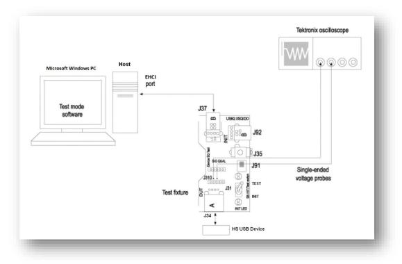
Figure 17: Equipment Setup for Resume Measurement
