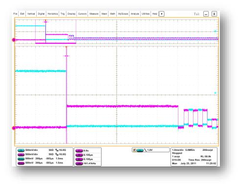
Figure 25: Device Reset from Suspend (EL\_28)
