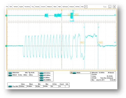
Figure 11: EL\_25 EOP in Device's Packet
