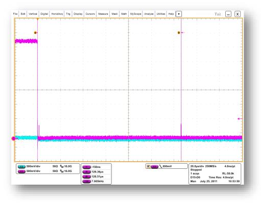
Figure 19: Device Resume to High-Speed (EL\_40)
