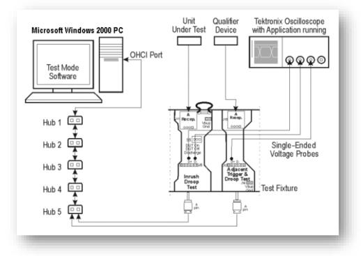
Figure 34: Equipment Setup for Full Speed Signal Quality Measurement
