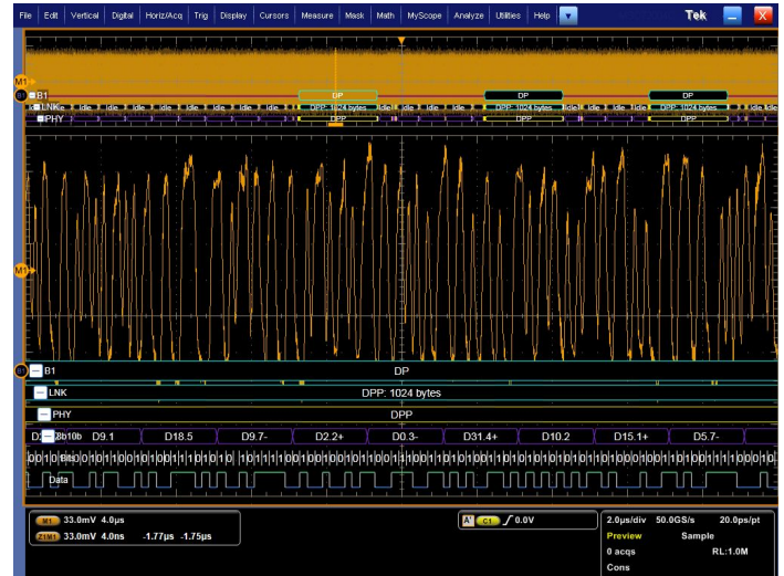
USB 3.0 bus display showing multiple layers simultaneously
