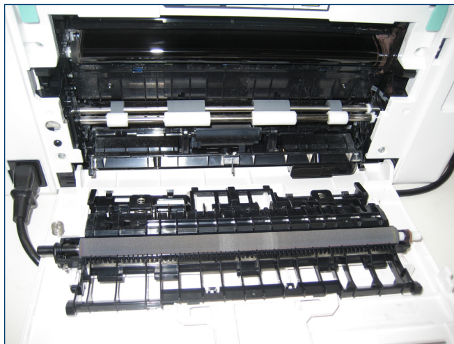
Exhibit K: No toner build-up on transfer rollers with Xerox cartridges.
