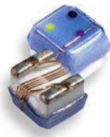
Due to accurate wire winding technology, these chip inductors are designed for filtering, impedance matching, resonance and choke circuits for RF designer. Both standard series custom designs are available.
