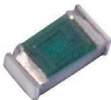
The TFL Series is designed for miniaturized devices, featuring low inductance, high precision and low loss. It allows for easy impedance matching for both RF and IF circuit designs as well as compact high frequency circuit designs
