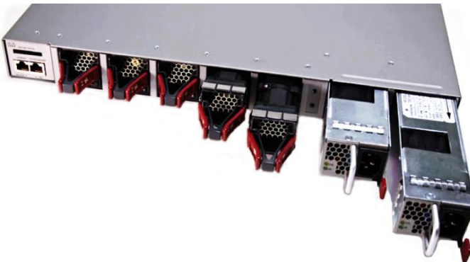
Figure 6. Redundant Fan and Power Supply
