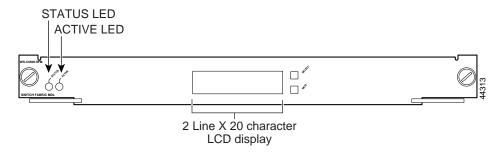
Two front-panel LEDs provide status information for the module and indicate whether the module is active. The STATUS LED functions are listed in Table 1-17 on page 1-29. (The ACTIVE LED is green when the module is operational and active, and is orange when the module is in standby mode.)
