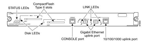
Figure 1-3 Supervisor Engine 32 (WS-SUP32-GE-3B) Front Panel Features
