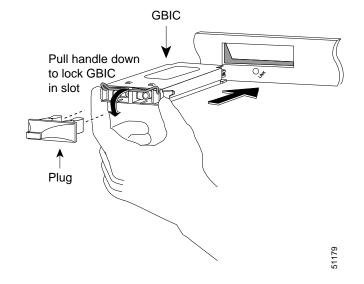
You can install the GBIC with the handle either up or down.
