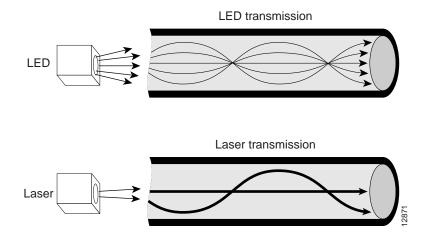
Lasers launch light in a more concentrated fashion. A laser transmitter couples light into only a fraction of the existing modes or optical pathways present in the fiber-optic cable. (See Figure 2-3.)
