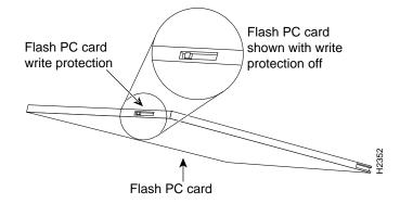
Use this procedure for installing and removing a Flash PC card:
