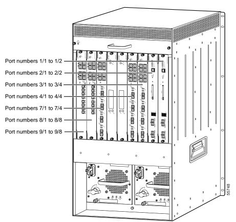
Figure 1-41 Cisco 7609 Router Port Address Examples
