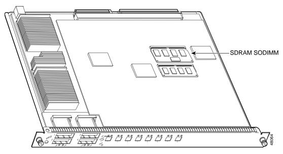
Step 5 Release the spring clips from the SODIMM that you want to remove, and release the SODIMM from the socket. (See Figure C-2.)
