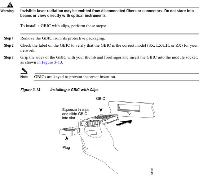
Step 4 Slide the GBIC through the flap covering the socket opening until you hear a click indicating the GBIC is locked into the slot.
