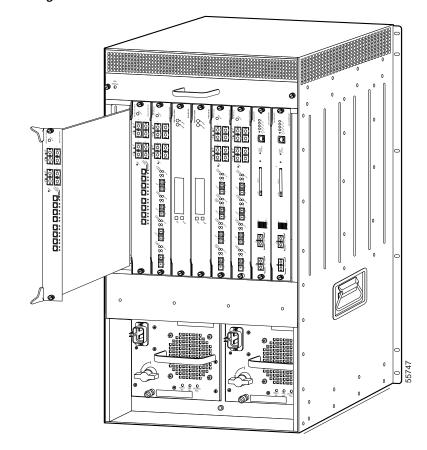
Figure 3-10 Installing a Module in the Cisco 7609 Router
