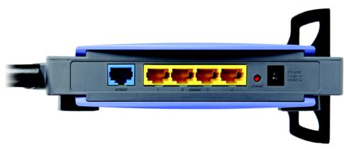
Figure 3-1: The Router's Back Panel
