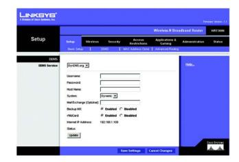
ddns: allows the hosting of a website, FTP server, or e-mail server with a fixed domain name (e.g., www.xyz.com) and a dynamic IP address.
