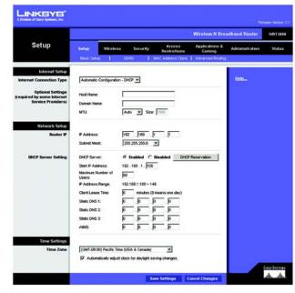
Figure 5-2: Setup Tab - Basic Setup (Automatic Configuration - DHCP)
