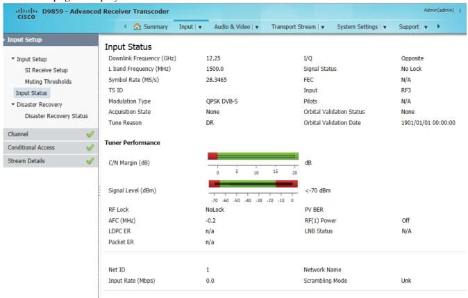
The **Current Input Status** area displays the same information shown in the **Input Setup** page. For more information on the parameters displayed, see *Setting up the RF Input* (on page 141).
