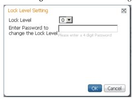
3 From the **Lock Level** drop-down list, choose the lock level that restricts access and prevents unauthorized changes to the transcoder settings (0, 1, 2, 3, or 4). The default setting is 0.
