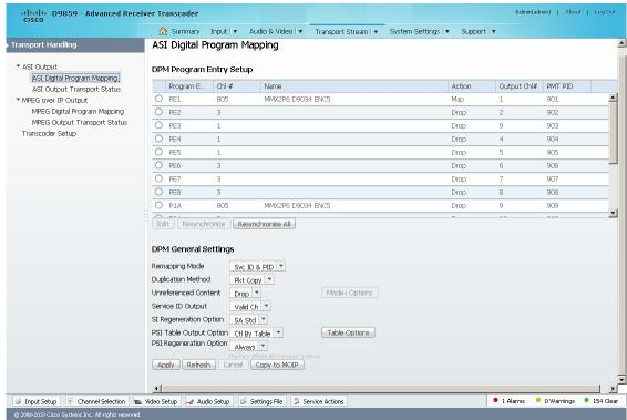
2 For each DPM **Program Entry**, it displays the input channel number (Chl #) and channel **Name**.
