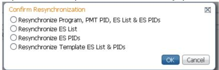
**2** Check whether you want to synchronize the PE output according to the services and then the PIDs assigned to each service, services only, PIDs only, or to synchronize using a template.
