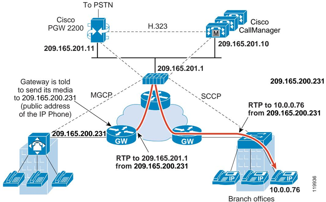
MGCP endpoints are physical or virtual sources and destinations for data. Media gateways contain endpoints on which the call agent can create, modify and delete connections to establish and control media sessions with other multimedia endpoints. Also, the call agent can instruct the endpoints to detect certain events and generate signals. The endpoints automatically communicate changes in service state to the call agent.
