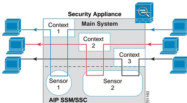
Figure 30-4 shows a single mode security appliance paired with multiple virtual sensors (in inline mode); each defined traffic flow goes to a different sensor.
