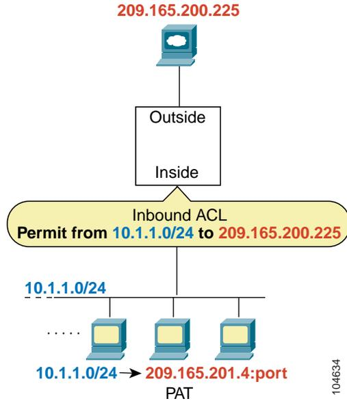
If you want to allow an outside host to access an inside host, you can apply an inbound access rule on the outside interface. You need to specify the translated address of the inside host in the access rule because that address is the address that can be used on the outside network. (See [Figure 21-3.](#))
