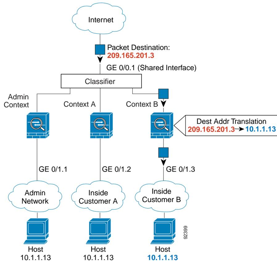
Note that all new incoming traffic must be classified, even from inside networks. Figure 11-3 shows a host on the Context B inside network accessing the Internet. The classifier assigns the packet to Context B because the ingress interface is Gigabit Ethernet 0/1.3, which is assigned to Context B.
