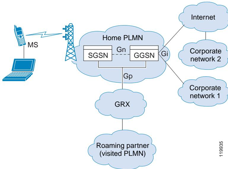
The UMTS is the commercial convergence of fixed-line telephony, mobile, Internet and computer technology. UTRAN is the networking protocol used for implementing wireless networks in this system. GTP allows multi-protocol packets to be tunneled through a UMTS/GPRS backbone between a GGSN, an SGSN and the UTRAN.
