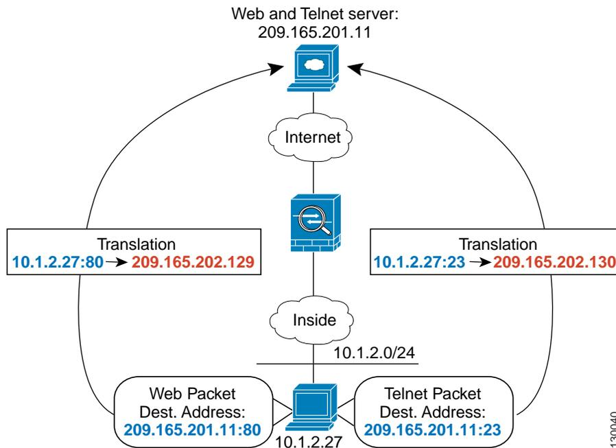
For policy static NAT, both translated and remote hosts can originate traffic. For traffic originated on the translated network, the NAT rule specifies the real addresses and the *destination* addresses, but for traffic originated on the remote network, the rule identifies the real addresses and the *source* addresses of remote hosts who are allowed to connect to the host using this translation.
