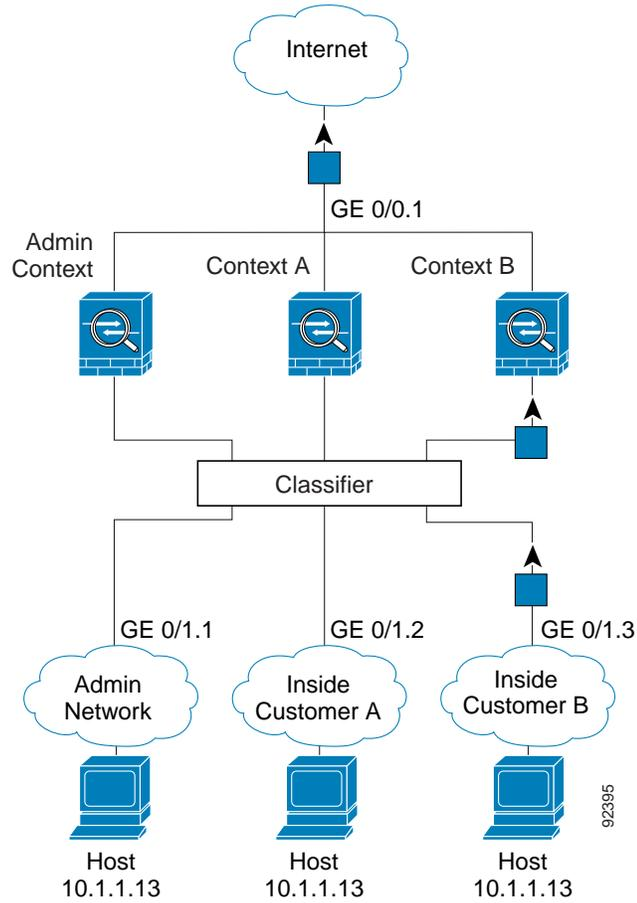
For transparent firewalls, you must use unique interfaces. [Figure 11-4](#) shows a host on the Context B inside network accessing the Internet. The classifier assigns the packet to Context B because the ingress interface is Gigabit Ethernet 1/0.3, which is assigned to Context B.
