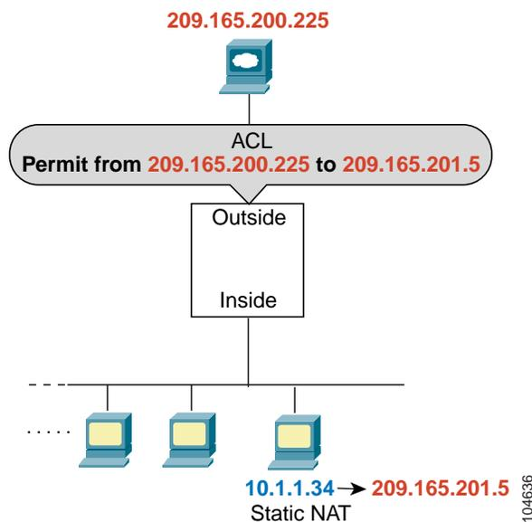
If you perform NAT on both interfaces, keep in mind the addresses that are visible to a given interface. In Figure 9-4, an outside server uses static NAT so that a translated address appears on the inside network.
