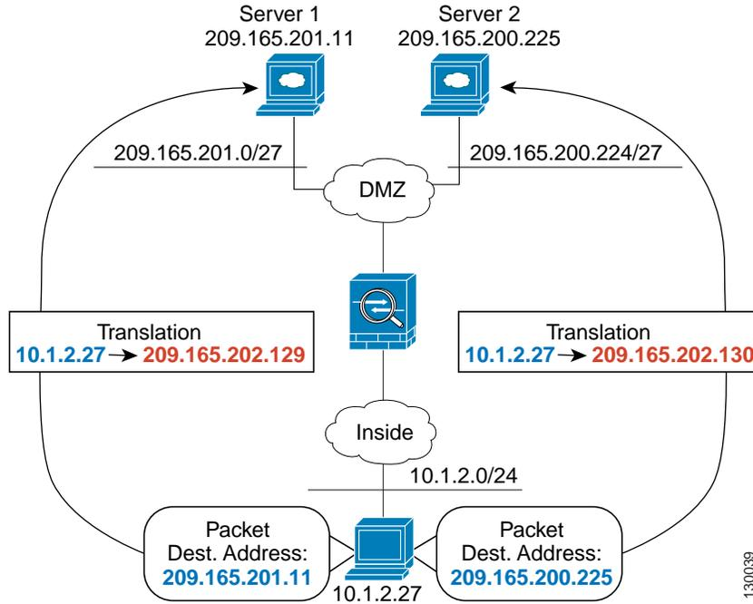
Figure 22-10 shows the use of source and destination ports. The host on the 10.1.2.0/24 network accesses a single host for both web services and Telnet services. When the host accesses the server for web services, the real address is translated to 209.165.202.129. When the host accesses the same server for Telnet services, the real address is translated to 209.165.202.130.
