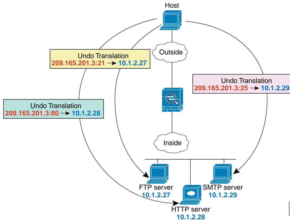
You can also use static PAT to translate a well-known port to a non-standard port or vice versa. For example, if inside web servers use port 8080, you can allow outside users to connect to port 80, and then undo translation to the original port 8080. Similarly, to provide extra security, you can tell web users to connect to non-standard port 6785, and then undo translation to port 80.
