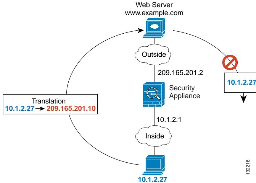
Figure 22-7 shows a remote host attempting to initiate a connection to a mapped address. This address is not currently in the translation table; therefore, the security appliance drops the packet.
