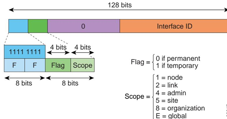
IPv6 nodes (hosts and routers) are required to join the following multicast groups:
