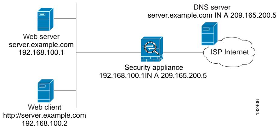
DNS rewrite also works if the client making the DNS request is on a DMZ network and the DNS server is on an inside interface.
