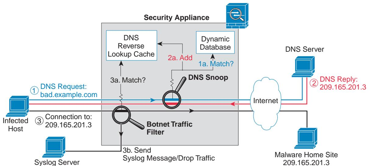
Figure 29-2 shows how the Botnet Traffic Filter works with the static database.
