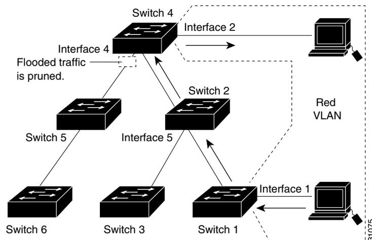
Enabling VTP pruning on a VTP server enables pruning for the entire management domain. VTP pruning takes effect several seconds after you enable it. By default, VLANs 2 through 1000 are eligible for pruning. VTP pruning does not prune traffic from pruning-ineligible VLANs. VLAN 1 is always ineligible for pruning; traffic from VLAN 1 cannot be pruned.
