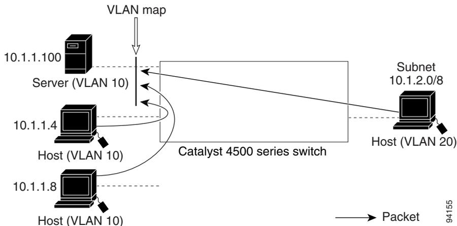
This procedure configures ACLs with VLAN maps to deny access to a server on another VLAN. The VLAN map `SERVER1_ACL` denies access to hosts in subnet 10.1.2.0/8, host 10.1.1.4, and host 10.1.1.8. Then it permits all other IP traffic. In Step 3, VLAN map `SERVER1` is applied to VLAN 10.
