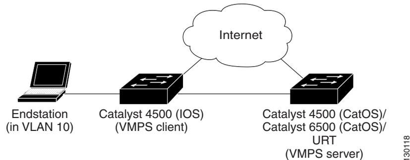
**Figure 10-6 Dynamic Port VLAN Membership Configuration**
