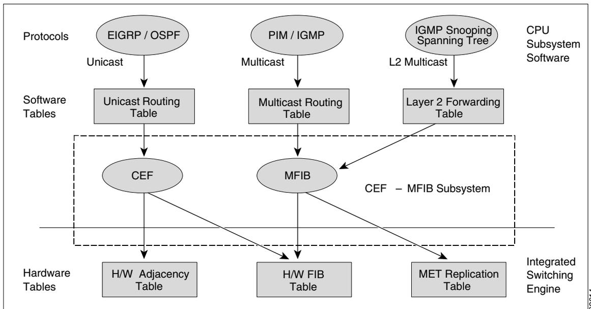
Like the CEF unicast routes, the MFIB routes are Layer 3 and must be merged with the appropriate Layer 2 information. The following example shows an MFIB route:
