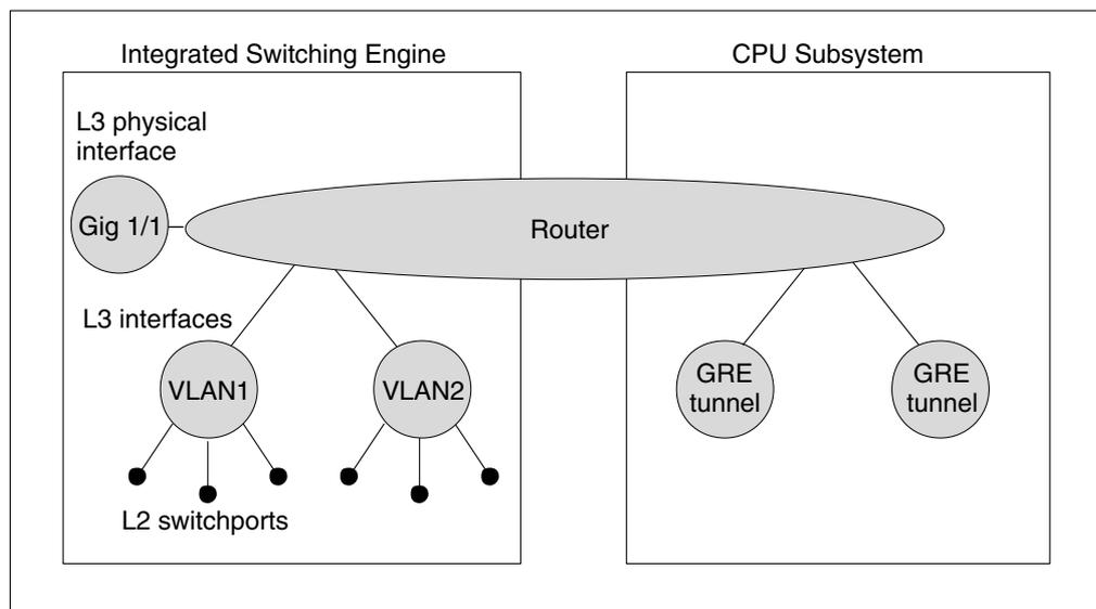
In the normal mode of operation, the Integrated Switching Engine performs inter-VLAN routing in hardware. The CPU subsystem supports generic routing encapsulation (GRE) tunnels for forwarding in software.
