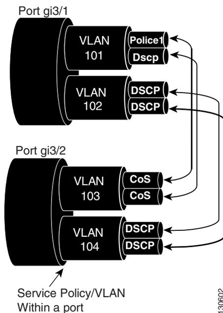
The following configuration file shows how to perform ingress and egress policing per VLAN using the policy-map P31\_QOS applied to port Gigabit Ethernet 3/1:
