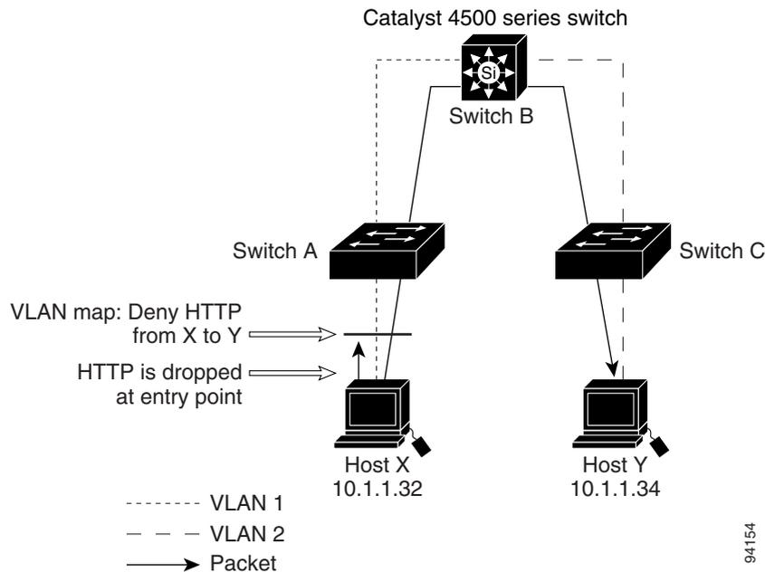
For example, if you do not want HTTP traffic to be switched from Host X to Host Y, you could apply a VLAN map on Switch A to drop all HTTP traffic moving from Host X (IP address 10.1.1.32) to Host Y (IP address 10.1.1.34) at Switch A and not bridge the traffic to Switch B. To configure this scenario, you would do the following:
