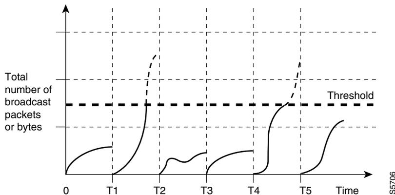
The broadcast suppression threshold numbers and the time interval combination make the broadcast suppression algorithm work with different levels of granularity. A higher threshold allows more broadcast packets to pass through.
