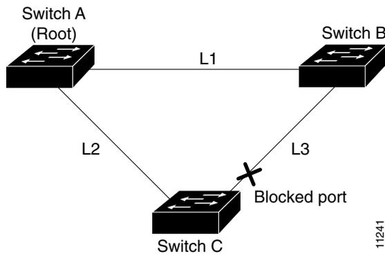
Next, assume that L1 fails. Switch A and Switch B, the switches directly connected to this segment, instantly know that the link is down. The blocking interface on Switch C must enter the forwarding state for the network to recover by itself. However, because L1 is not directly connected to Switch C, Switch C does not start sending any BPDUs on L3 under the normal rules of STP until the time defined by the Max Age setting has expired.
