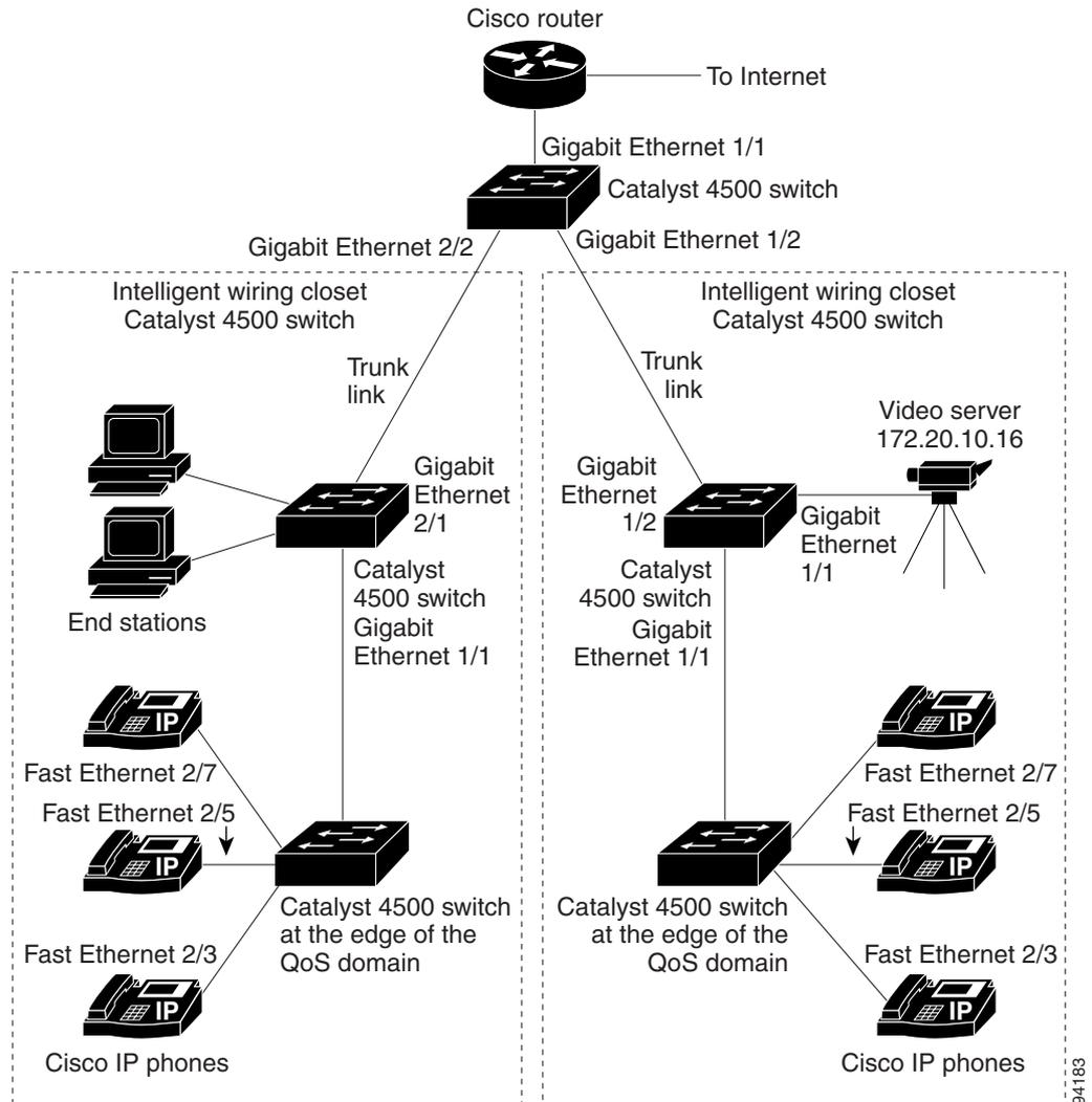
The intelligent wiring closets in [Figure 27-5](#) are composed of Catalyst 4500 switches. The object of this example is to prioritize the VoIP traffic over all other traffic. To do so, enable auto-QoS on the switches at the edge of the QoS domains in the wiring closets.
