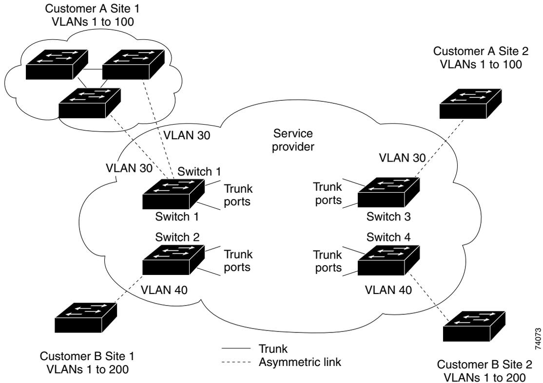
**Figure 18-5 Layer 2 Network Topology without Proper Convergence**
