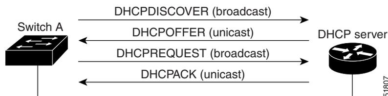
The client, Switch A, broadcasts a DHCPDISCOVER message to locate a DHCP server. The DHCP server offers configuration parameters (such as an IP address, subnet mask, gateway IP address, DNS IP address, lease for the IP address, and so forth) to the client in a DHCPOFFER unicast message.
