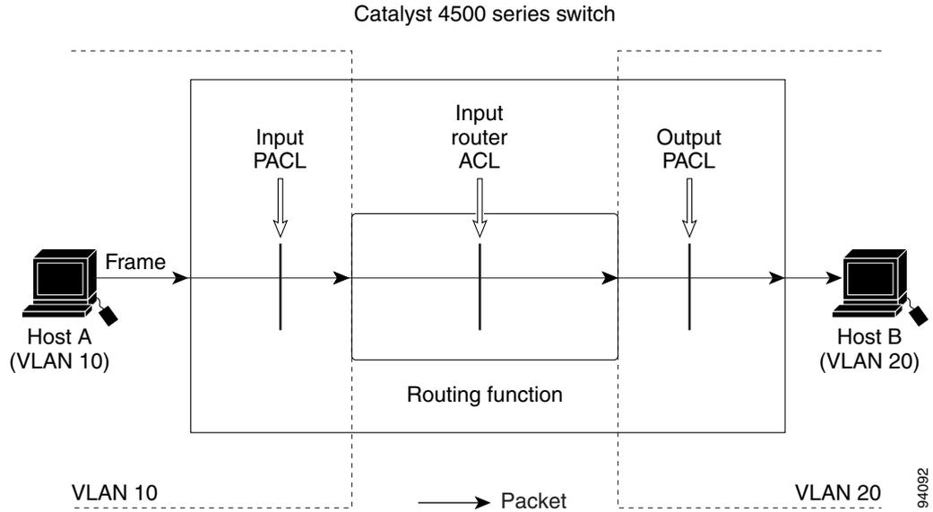
If the interface access group mode is prefer port, then only the input PACL is applied on the ingress traffic from Host A. If the mode is prefer vlan, then only the input Router ACL is applied to ingress traffic from Host A that requires routing. If the mode is merge, then the input PACL is first applied to the ingress traffic from Host A, and the input Router ACL is applied on the traffic that requires routing.
