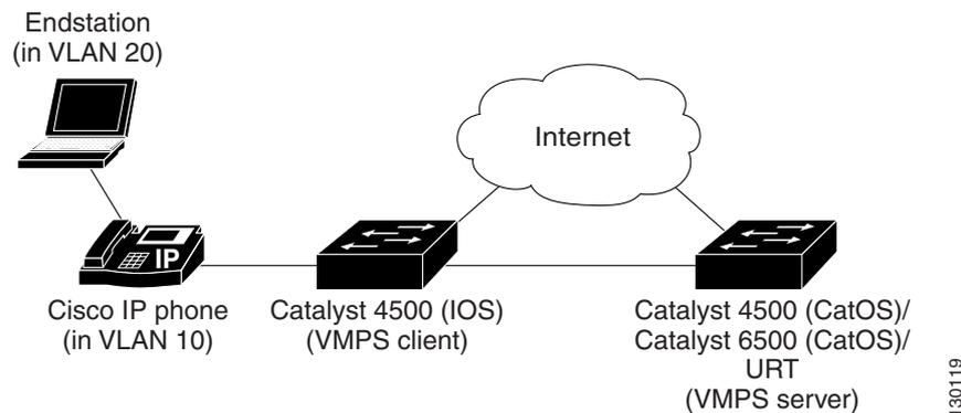
In the following procedure, the Catalyst 4000 and Catalyst 6000 series switches (running CatOS) are the VMPS servers. Use this procedure to configure the Catalyst 4500 series switch clients in the network:
