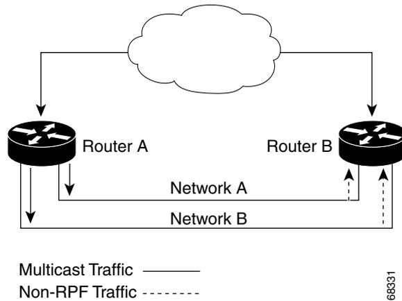
In this kind of topology, only Router A, the PIM designated router (PIM DR), forwards data to the common VLAN. Router B receives the forwarded multicast traffic, but must drop this traffic because it has arrived on the wrong interface and fails the RPF check. Traffic that fails the RPF check is called non-RPF traffic.
