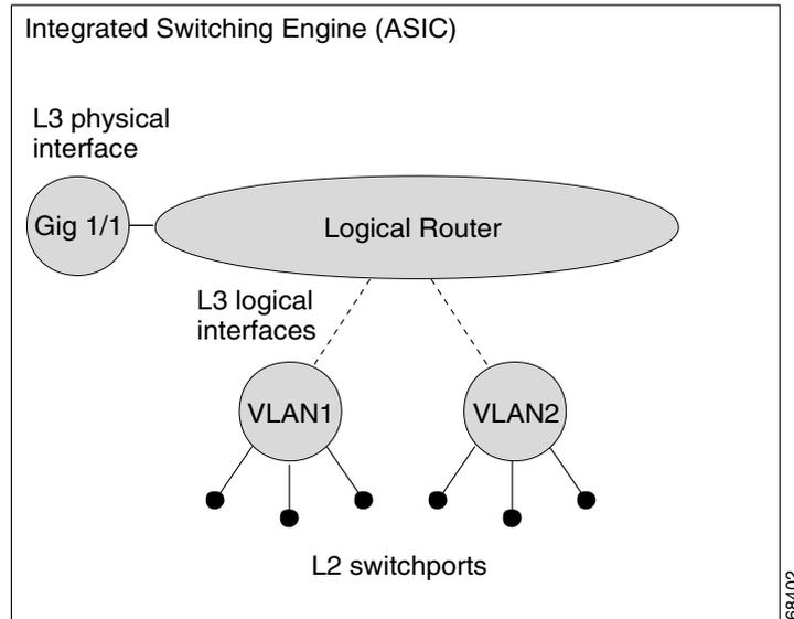
The Integrated Switching Engine performs inter-VLAN routing on logical Layer 3 interfaces with the ASIC hardware. The ASIC hardware also supports a physical Layer 3 interface that can be configured to connect with a host, a switch, or a router.
