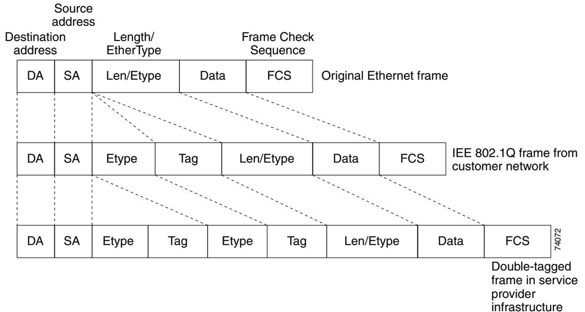
When the packet enters the trunk port of the Service Provider egress switch, the metro tag is again stripped as the switch processes the packet. However, the metro tag is not added when the packet is sent out the tunnel port on the edge switch into the customer network. The packet is sent as a normal 802.1Q-tagged frame to preserve the original VLAN numbers in the customer network.
