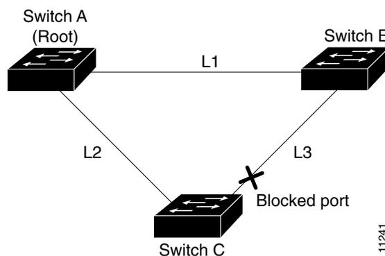
If Switch C detects a link failure on the currently active link L2 on the root port (a direct link failure), UplinkFast unblocks the blocked port on Switch C and transitions it to the forwarding state without going through the listening and learning states, as shown in Figure 14-3. This switchover takes approximately one to five seconds.
