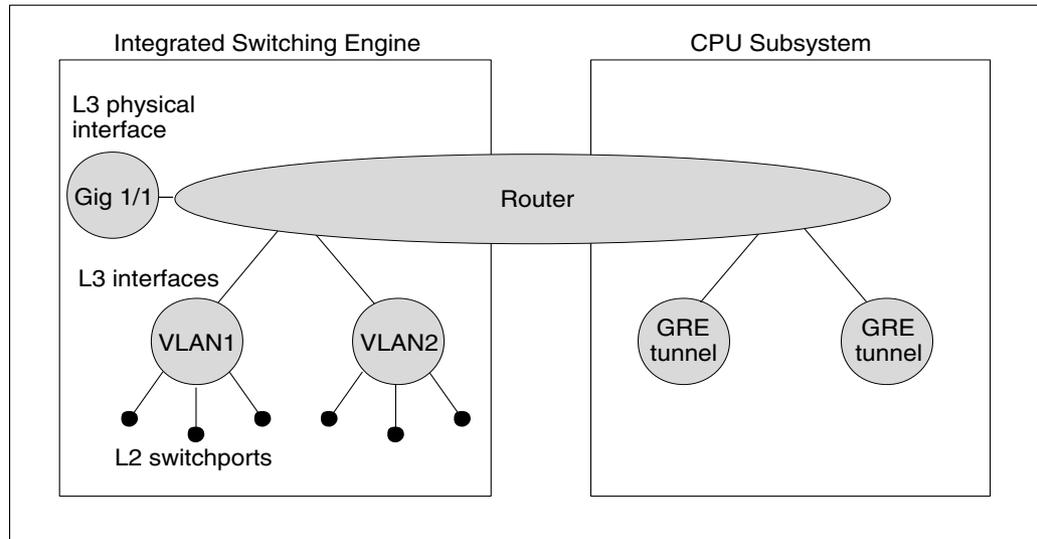
The Integrated Switching Engine performs inter-VLAN routing in hardware. The CPU subsystem software supports Layer 3 interfaces to VLANs that use Subnetwork Access Protocol (SNAP) encapsulation. The CPU subsystem software also supports generic routing encapsulation (GRE) tunnel.
