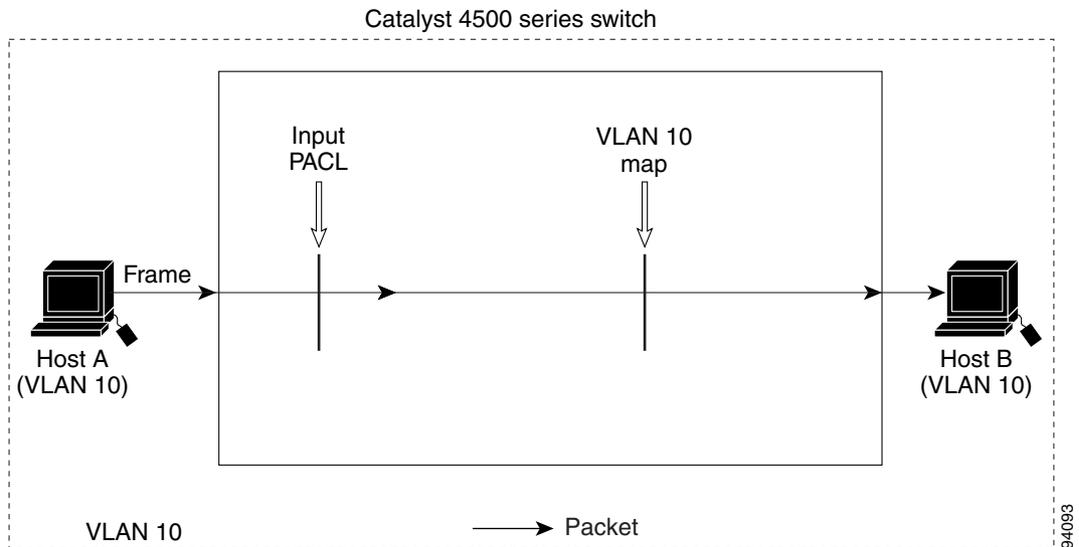
If the interface access group mode is `prefer port`, then only the input PACL is applied on the ingress traffic from Host A. If the mode is `prefer vlan`, then only the VACL is applied to the ingress traffic from Host A. If the mode is `merge`, the input PACL is first applied to the ingress traffic from Host A, and the VACL is applied on the traffic.
