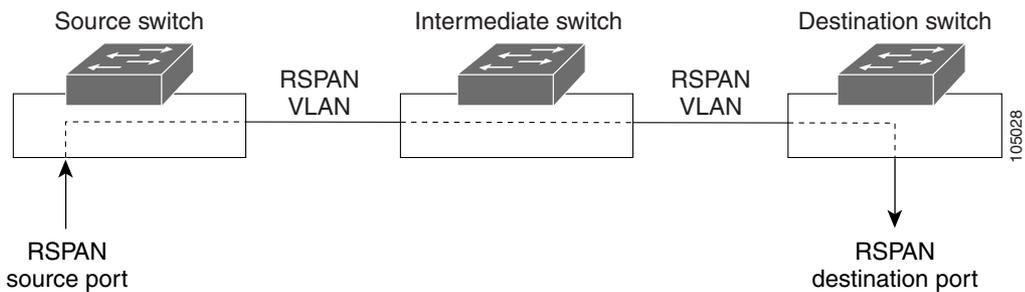
SPAN and RSPAN do not affect the switching of network traffic on source ports or source VLANs; a copy of the packets received or sent by the sources is sent to the destination. Except for traffic that is required for the SPAN or RSPAN session, by default, destination ports do not receive or forward traffic.
