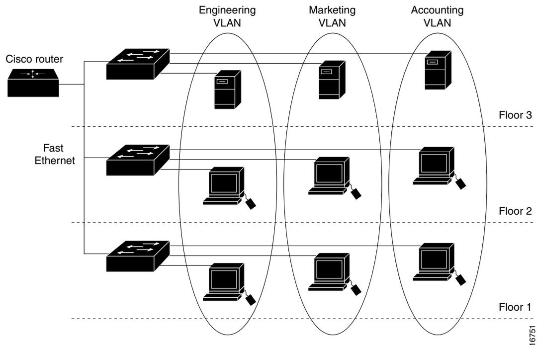
VLANs are often associated with IP subnetworks. For example, all of the end stations in a particular IP subnet belong to the same VLAN. Traffic between VLANs must be routed. You must assign LAN interface VLAN membership on an interface-by-interface basis (this is known as interface-based or static VLAN membership).
